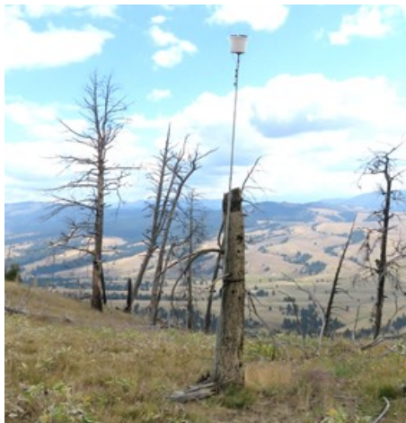
Photo by Kate Stone A directional microphone hides inside this bucket on Sula Peak.
